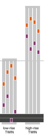
elevator cabins can move independently from one another. Passengers in the upper zone of the building enter the TWIN elevator cabin via the upper access level. The same principle applies to the lower elevator cabin and the lower zone of the building. After the morning peak traffic, the virtual zones are "opened" and both TWIN elevator cabins serve the complete shaft.
