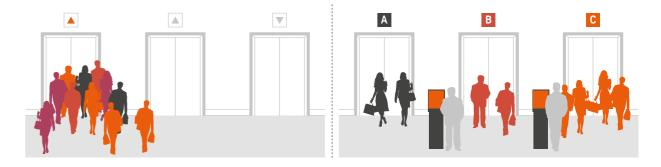
analyses the request – gauging traffic demand and grouping passengers based on similarity of destination. This leads to less crowding, fewer stops and a more efficient use of available elevator capacity.
