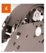
Automatic engagement of the safety gear In the unlikely event that the first three safety stages fail, the safety gears of both the elevator cabins are activated. It is not possible for the elevator cabins to make contact.
