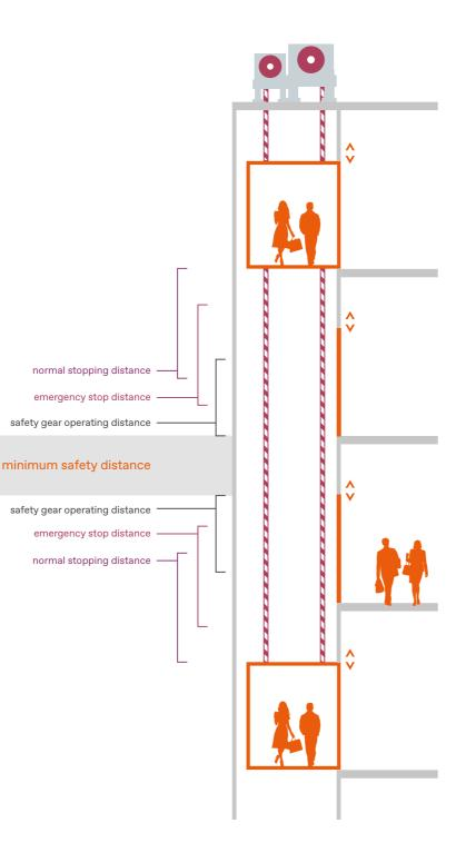
The key to the system's safety is that the cabins always operate at a minimum safety distance.
